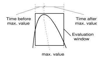
As the oscillation will be curtailed on the end of the frame, this gives rise to errors in the evaluation. These errors can be compensated for by computer, using various methods. These methods are the Hamming, Hanning and Blackman methods. In general the Hamming method will be used.
