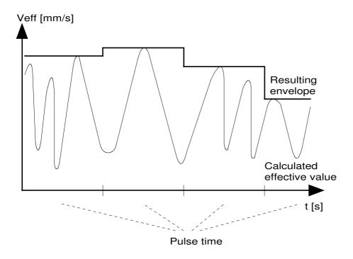
The registration of the KB-value measurement (DIN 4150) will be exactly the same. In this case however, the oscillation velocity of the envelope as well as the vectors will not be given in mm/s i.e. no measuring units will be used.
